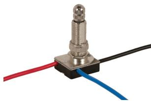
**80-1365** - 3-Way Metal Rotary Switch, Metal Bushing, 2 Circuit, 4 Position(L-1, L-2, L1-2, Off). Rated: 6A-125V, 3A-250V
